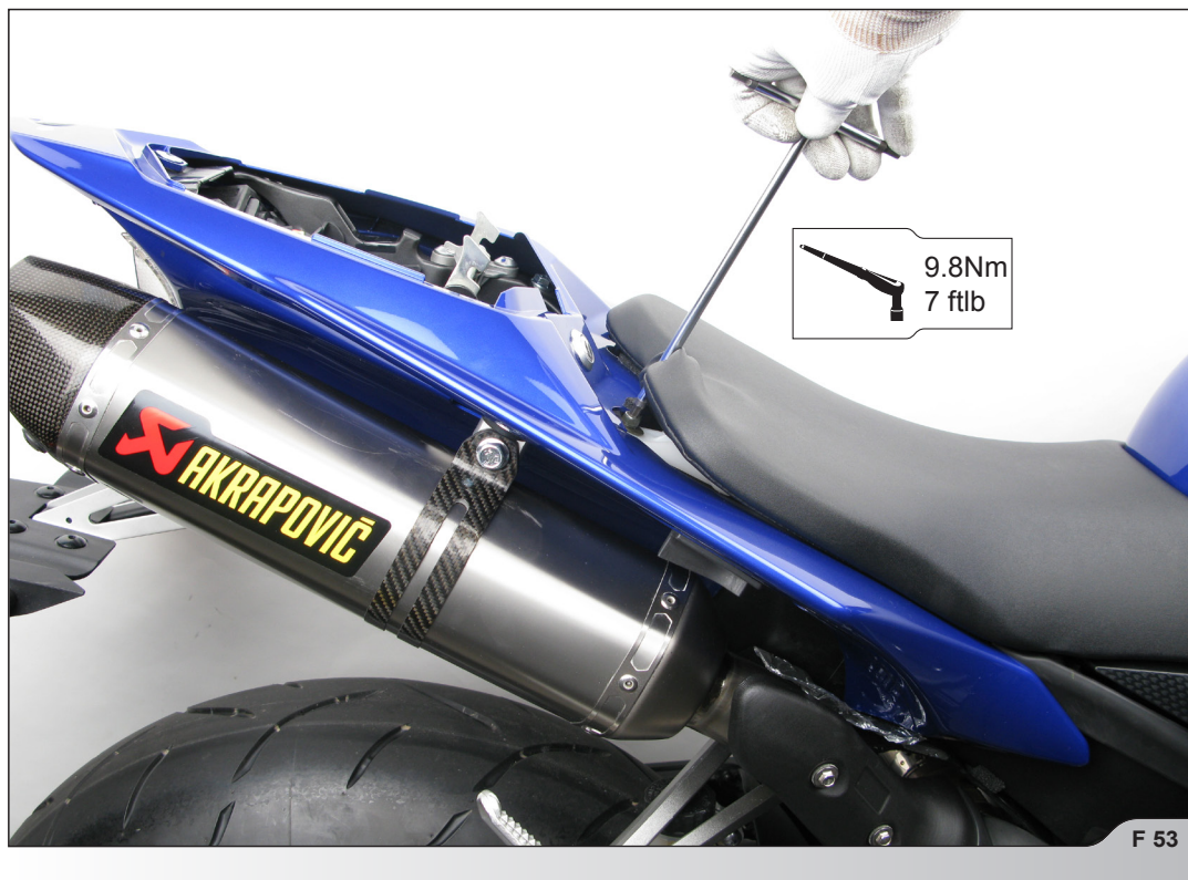
14. Position of the correctly installed Akrapovic SLIP-ON system (F 54).
